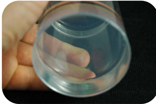
Figure 6. Concentrated haze observed in MS solidified using common food grade gellan Gum. Note darker haze toward bottom of gel with clearing toward top of gel. Gel solidified throughout.
